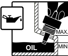
**NOTE:** When filling the crankcase, the oil flows very slowly into the pump. If the oil is added too quickly, it will overflow and appear to be full.
